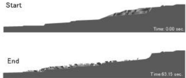
Figure 6. Result of the Run 05 in DDA (divided into the large blocks).
