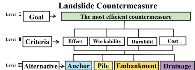
Figure 1 Example of AHP model
