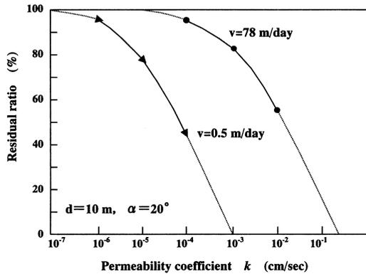
Fig. 7 Groundwater residual ratio versus permeability coefficient for different values of reservoir level draw-down speed
