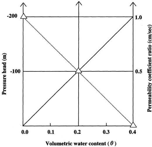
Fig. 2 Relationships of volumetric moisture contents, permeability and pore water pressure
