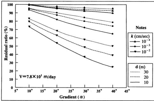
Fig. 4 Groundwater residual ratio versus slope gradient for different values of permeability coefficient and layer thickness at  $v=7.8 \times 10^1$  m/day
