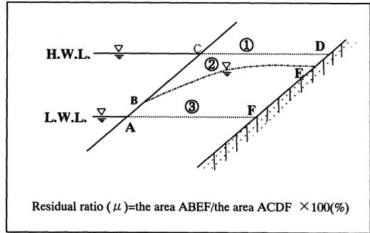
Fig. 3 Method of determining the groundwater residual ratio ( $\mu$ )
