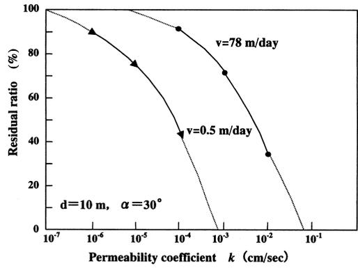
Fig. 6 Groundwater residual ratio versus permeability coefficient for different values of reservoir level draw-down speed
