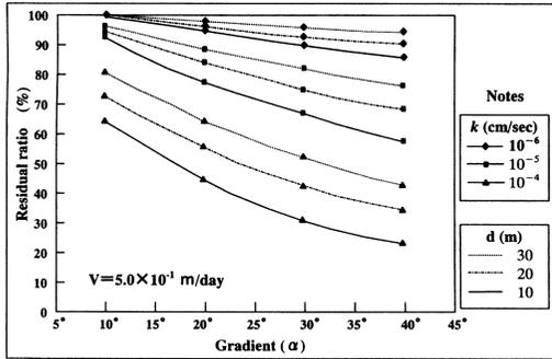
Fig. 5 Groundwater residual ratio versus slope gradient for different values of permeability coefficient and layer thickness at  $v=5.0 \times 10^1$  m/day
