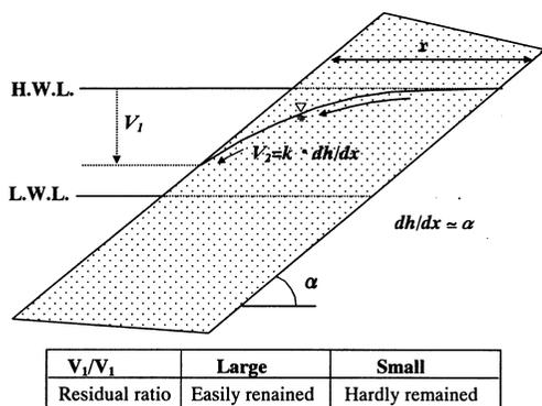
Fig. 8 Conceptual diagram of seepage flow model
